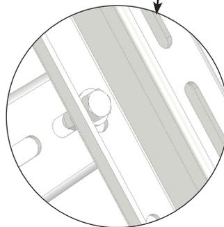
3. Adjust the tilt of the panel, then tighten the tilt plate nuts to 12 ft-lbs.
