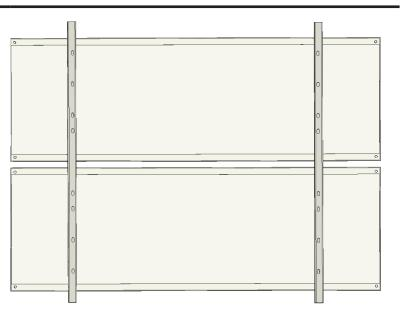
3. Secure the rails with a bolt, lock washer and hex nut in each of the PV mounting holes.
