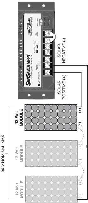
Figure 6. Solar input wiring.
