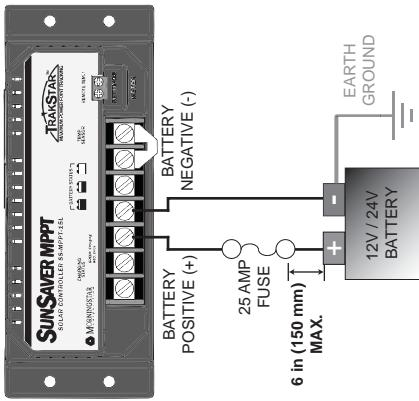
Figure 5. Battery wiring.
