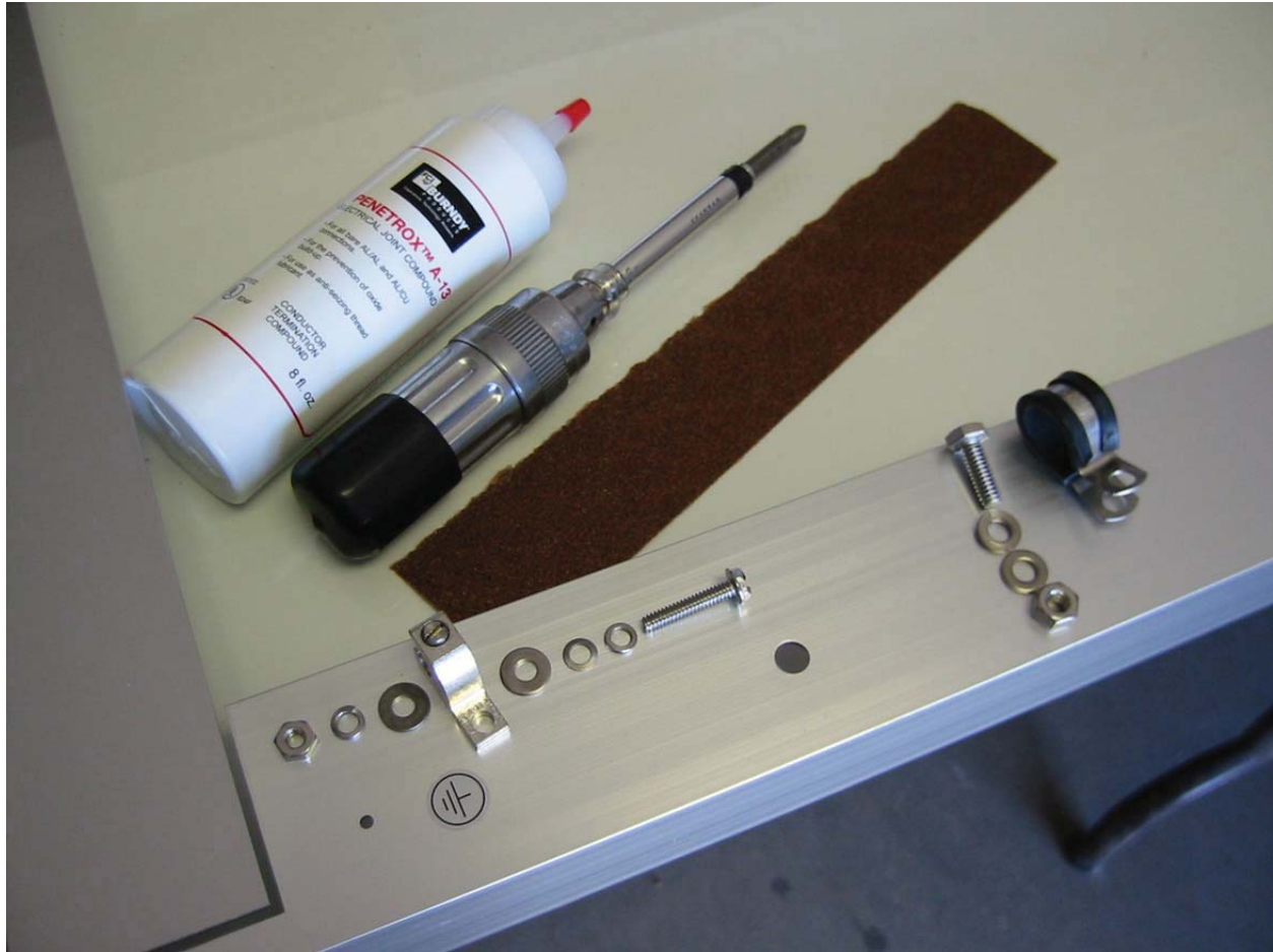
Figure G-2. Connecting Tin-plated Copper Lug to Aluminum
