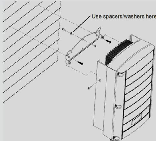
**5** Optionally, secure the Safety Switch bracket to the wall:
