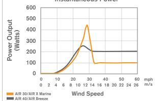
\*Factors affecting turbine output include site turbulence, elevation and air temperature
