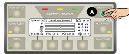
4. Press the **<Detail>** soft key **E** when the desired event is highlighted in the list. This opens the **Event History Detail** screen.
