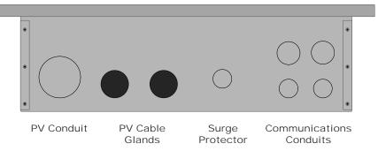
NOTE: Any installed devices must be liquid-tight to sustain the combiner's environmental rating.
