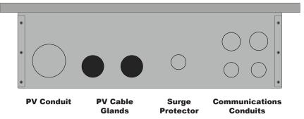
**NOTE**: Any installed devices must be liquid-tight to sustain the combiner's environmental rating.
