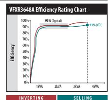
**Typical Efficiency Rating**Real world efficiency with variable loads **VFXR3648A**: 93%
