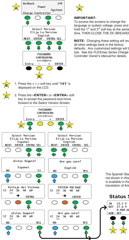
hold the 1<sup>st</sup> and 3<sup>rd</sup> soft key at the same time. THEN CLOSE THE DC BREAKERS.
