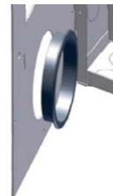
Figure 11, Installing 3.5" Grommet in the Door
