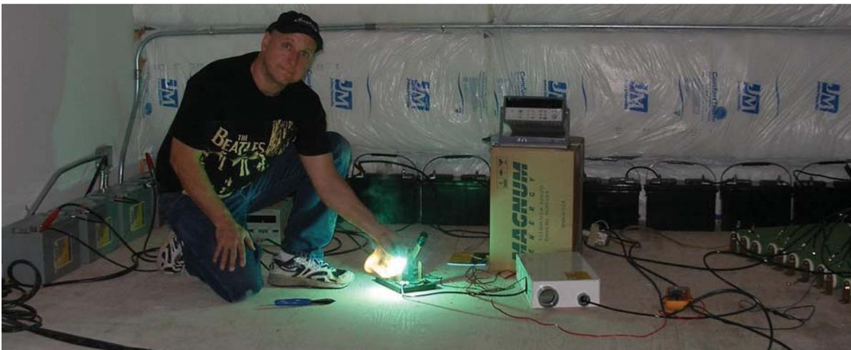
Pictured above, boB breaking 165VDC at 99 amps for the first test. This arc is the same arc that our little breaker must deal with internally. The arc is not only blinding, but also extremely hot. Pretty amazing huh! I also discovered the hard way that getting shocked with 165VDC feels pretty much the same as getting shocked with 120VAC.
