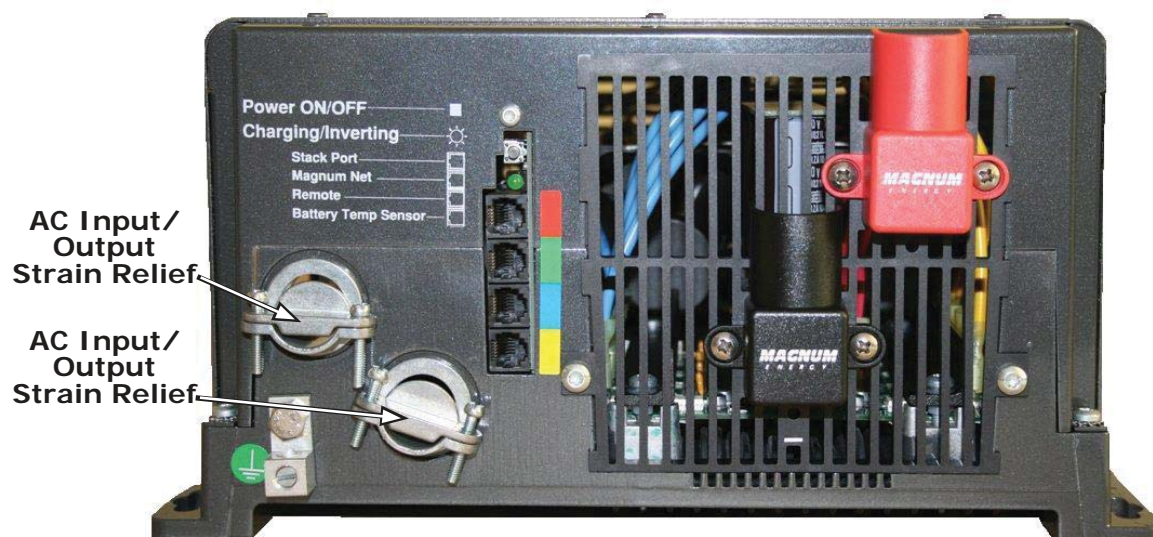
Figure 2-8, RD Series Inverter/Charger - AC Wiring
