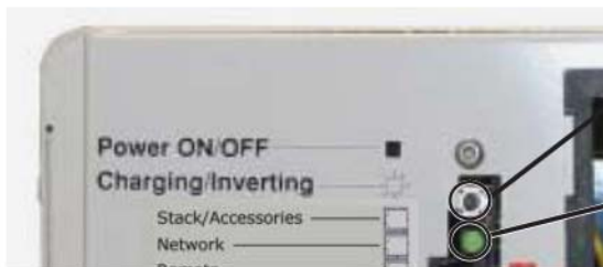
Figure 6-1, Performing an Inverter Reset
