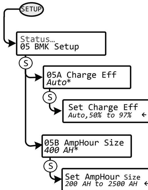
Figure 4-3, ME-ARC50 SETUP Menu Map (Displays w/BMK Settings)
