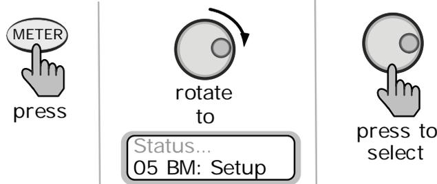
**Figure 3-1, Accessing the Charge Efficiency Menu Item (ME-RC50)**
