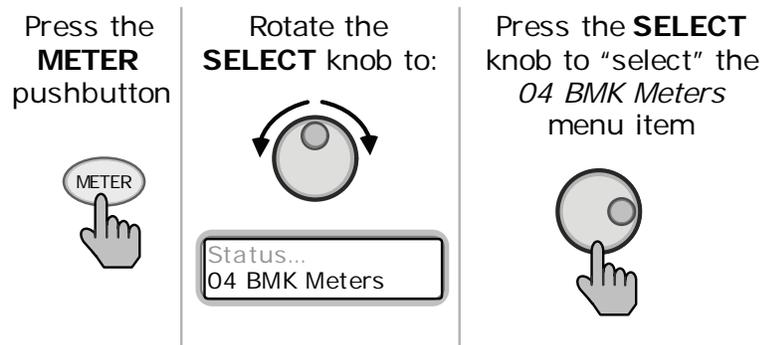
**Figure 4-5, Accessing the METER Menu Items (ME-ARC50)**
