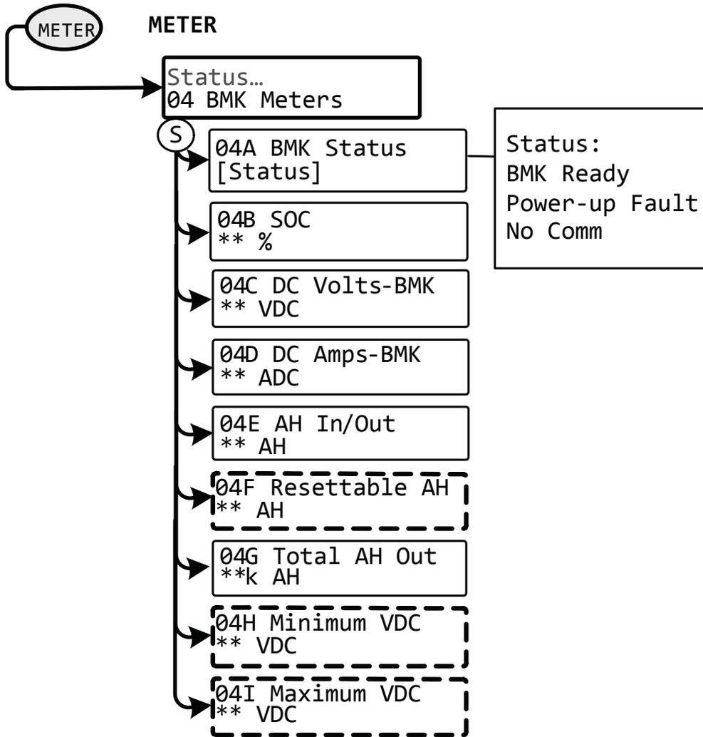
Figure 4-4, ME-ARC50 METER Menu Map (Displays w/BMK Settings)
