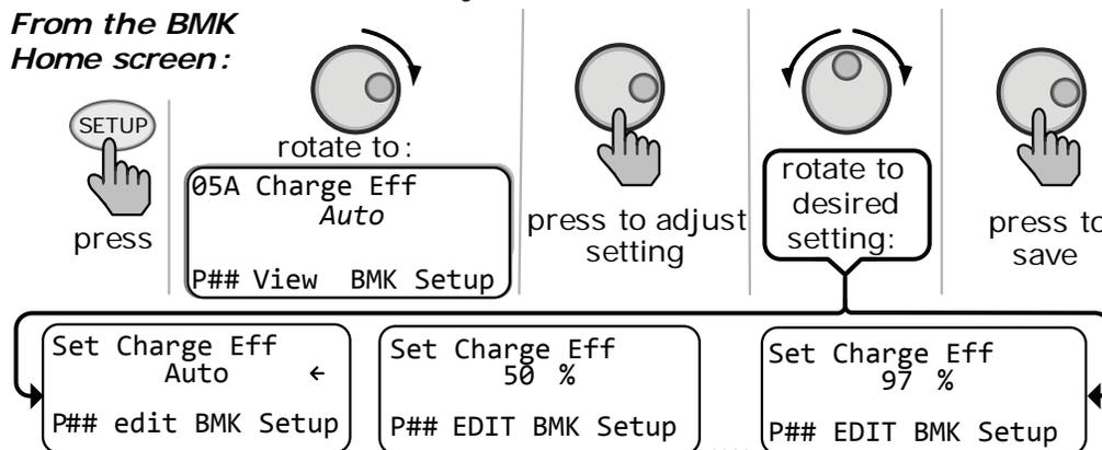
**Figure 5-2, Adjusting the Charge Efficiency Setting (ME-RTR)**
