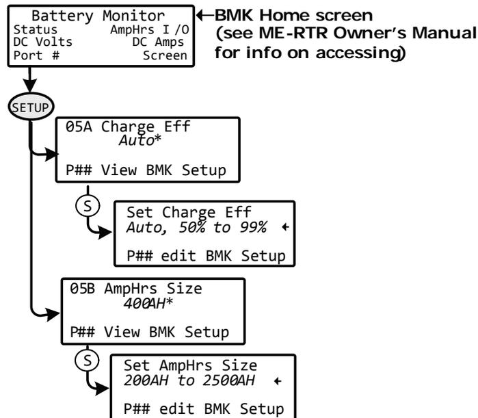
*Figure 5-3, ME-RTR SETUP Menu Map (Displays w/BMK Settings)*
