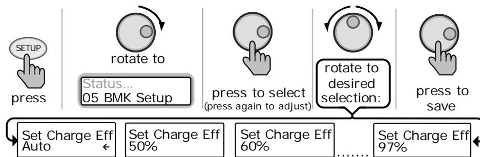
**Figure 4-2, Adjusting the Charge Efficiency Setting (ME-ARC50)**
