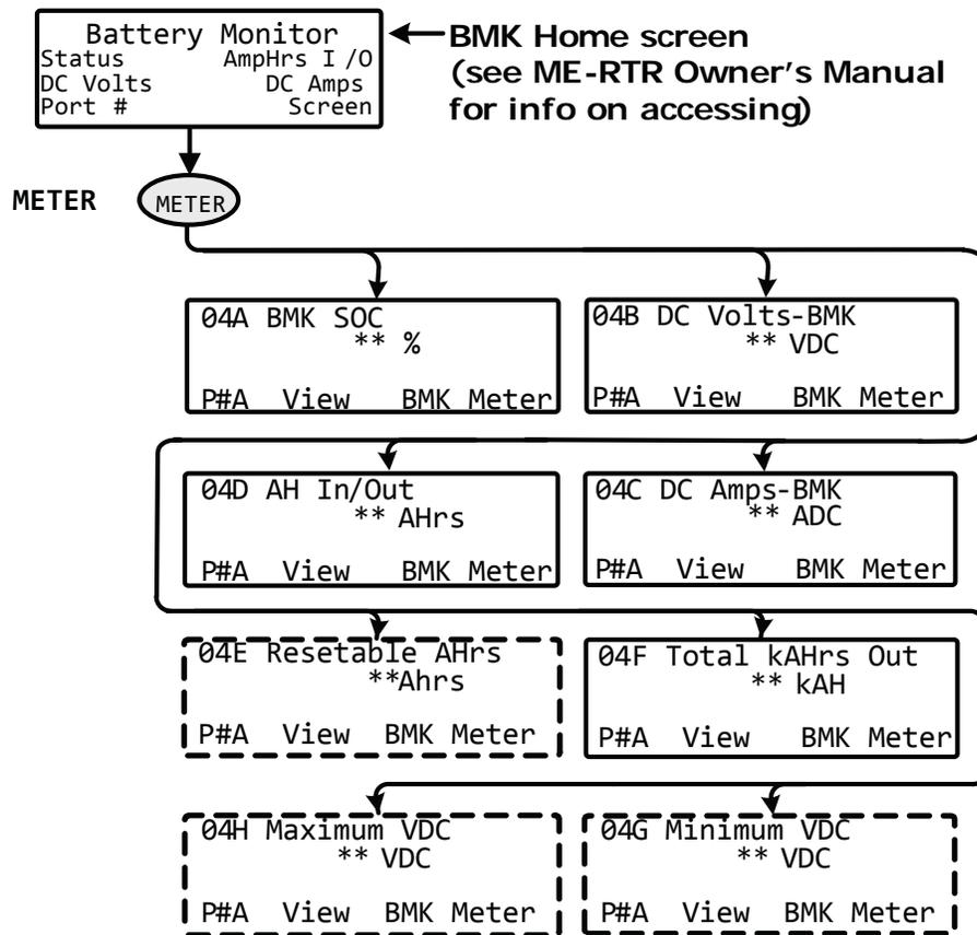
Figure 5-4, ME-RTR METER Menu Map (Displays w/BMK Settings)
