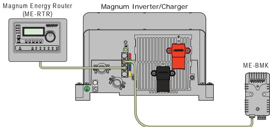
*Figure 2-7, BMK and Router w/ Separate Connections to Inverter*
