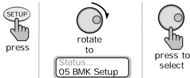
**Figure 4-1, Accessing the Charge Efficiency Menu Item (ME-ARC50)**
