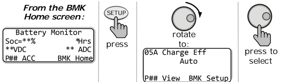
**Figure 5-1, Accessing the Charge Efficiency Menu Item (ME-RTR)**
