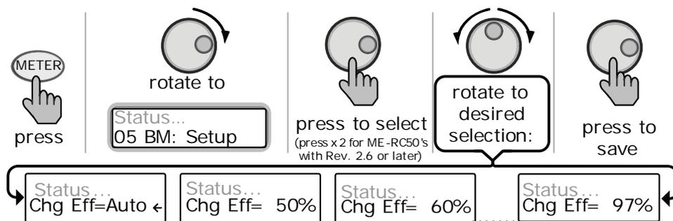
**Figure 3-2, Adjusting the Charge Efficiency Setting (ME-RC50)**
