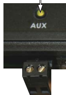
Aux Relay LED Indicator
