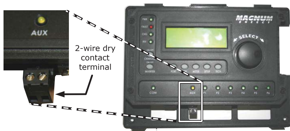
Figure 2-13, Wiring the Auxiliary Relay
