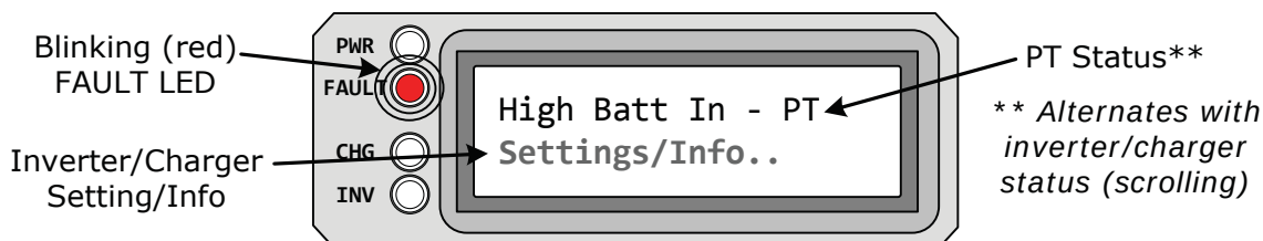
Figure 10-9, PT Controller Fault Message (Example)
