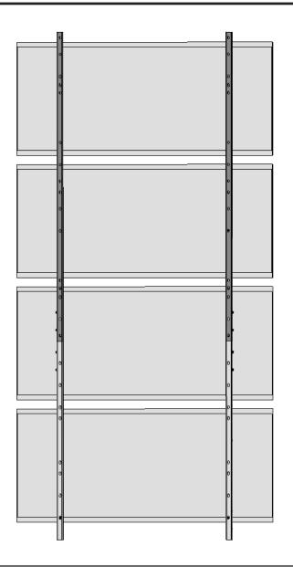
3. Secure the rails with a bolt, lock washer and hex nut in each of the PV mounting holes.
