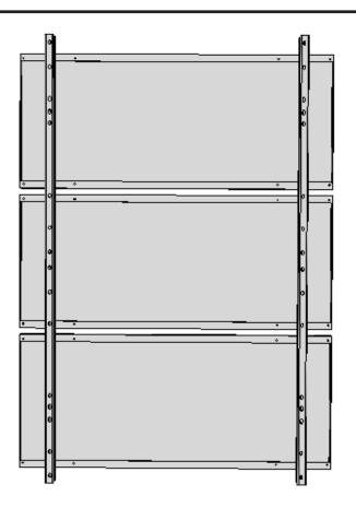
3. Secure the rails with a bolt, lock washer and hex nut in each of the PV mounting holes.
