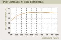
The typical change in module efficiency at an irradiance of 200 W/m² in relation to 1000 W/m² (both at 25  $^{\circ}$ C and AM 1.5 G spectrum) is -3 % (relative).
