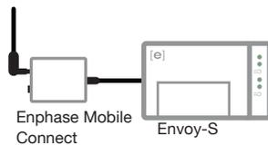
Within three minutes the Network Communications LED lights solid green, indicating a successful connection to Enlighten. If the Network Communications LED remains off or lights solid amber, see *Troubleshooting* in the *Enphase Mobile Connect Installation Guide*.
