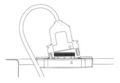
b. Cover any unused connectors with sealing caps. Listen for two clicks as the connectors engage. See notes in Step Details on back.
