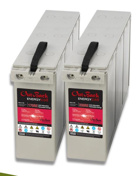
The EnergyCell RE valve regulated lead acid battery is designed for high power density and renewable energy cycling applications. Absorbed Glass Matt (AGM) technology for efficient gas recombination of up to 99% and freedom from electrolyte maintenance. The EnergyCell RE also features low profile terminals with threaded copper alloy inserts providing reduced maintenance and increased safety.
