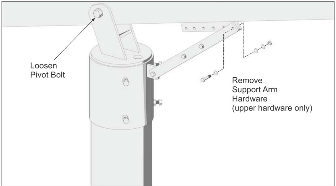
*Figure 7-1: Preparing to Adjust the Tilt Angle*
