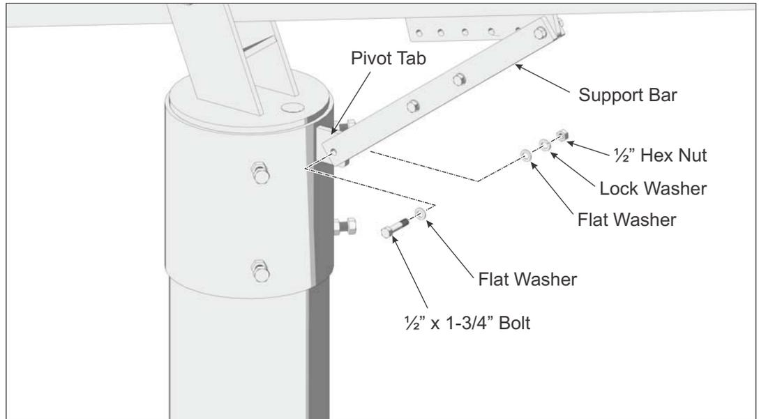
Figure 2-3: Securing Support Bar to Mounting Sleeve
