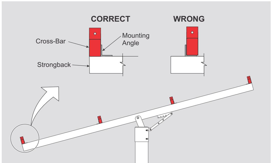
Figure 3-1: Cross-Bar Positioning relative to Mounting Angles
