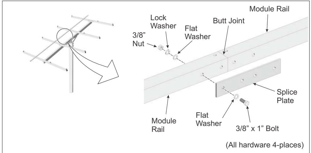
Figure 4-4: Attaching the Splice Plate to Module Rails
