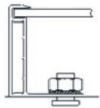
Example A: Bolting (INTERTEK and CSA qualified)
