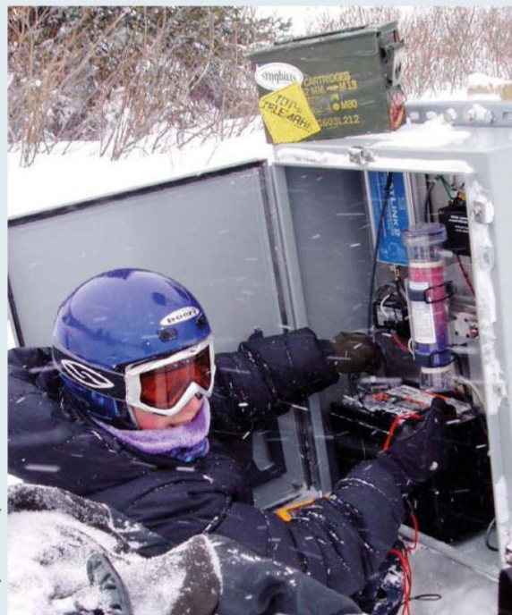
It's a cold snowmobile ride to maintain this remote data-monitoring system powered by a PV system with an AGM battery.
