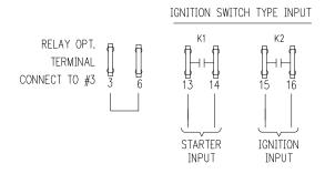
EMERGENCY SHUTDOWN "KILL" SWITCH WIRING (IGNITION)
