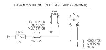
The K1 relay provides a continuous run signal for generators requiring a "maintained" start signal. The K2 relay provides a momentary "stop" signal until the generator AC Hz has dropped to zero. For GSCM-mini operational sequence details see Page 4, Section - 2
