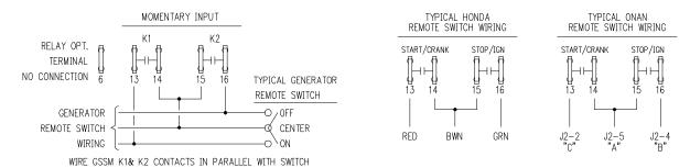
The K1 relay is used to switch the start/crank input which is looking for a momentary signal and opens when the generator has reached 50Hz, or half speed. The K2 relay provides a momentary "stop" signal until the generator AC Hz has dropped to zero. For GSCM-mini operational sequence details see Page 4, Section - 1
