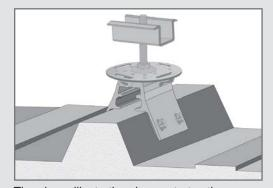
The above illustration demonstrates the RibBracket with the S-5-PV Kit attached.
