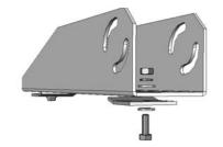
2. Repeat step 1 attaching the remaining clamp to the other slot on the arm.
