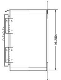
Brushed Aluminum (Cooler than steel) Lightweight and Durable NEMA 3R Stainless Steel Hinge and Hardware
