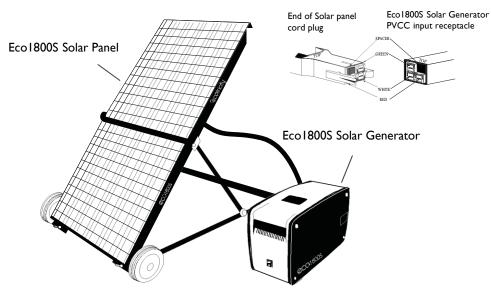
Cover the Eco1800S Solar Panel with an opaque sheet such as a sheet or blanket to reduce it's output to zero volts. Then follow instructions 11-2 to disassemble the Eco1800S Solar Panel.
