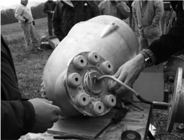
Fig. 11 Placing vibration isolators
