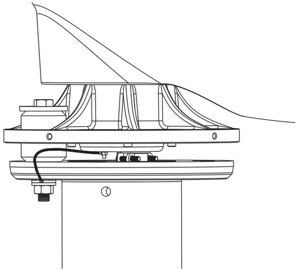
Fig. 5 Proper grounding of the yaw connection
