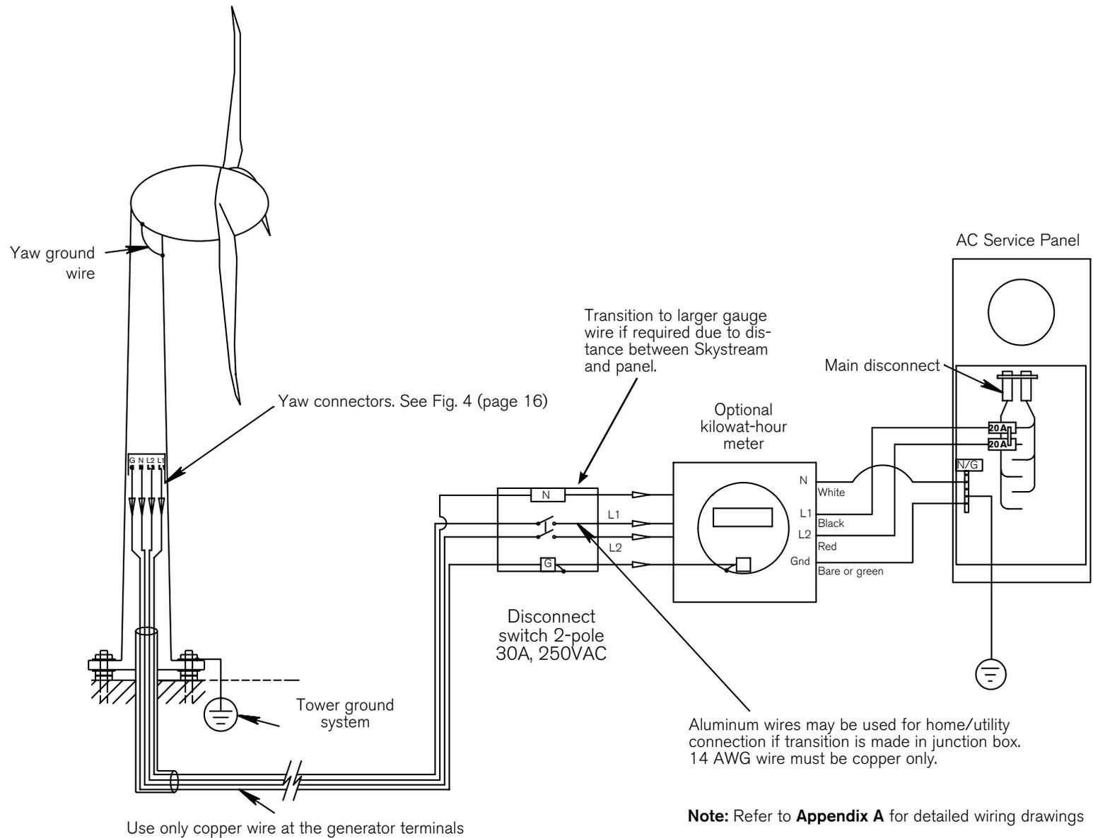
Fig. 3 Wiring diagram, 240V, 60Hz, split phase.
